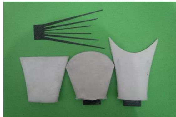
Figure 7 Fin made of silicon rubber and carbon fiber reinforcement
