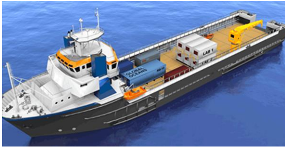
Figure 1 Project-configured OSV with labs, storage, on-deck accommodations & operational support
