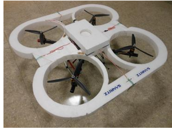
Figure 11 Test quad rotor helicopter with plastic bottle holder
