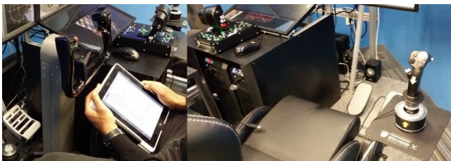
Figure 5 Pilot seat with the column yoke, co-pilot seat with the joystick
