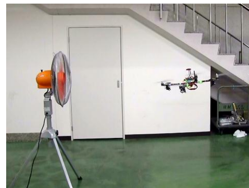
Figure 18 Scene of crosswind test
