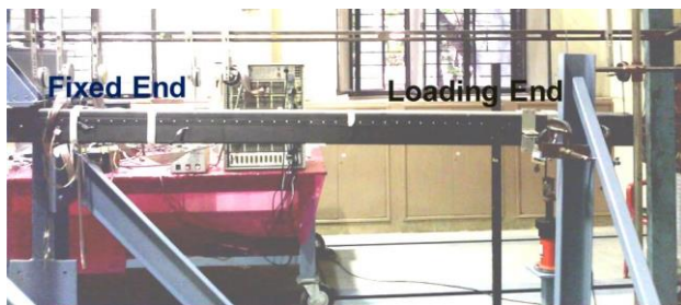
Figure 5 Experimental setup for boom static testing
