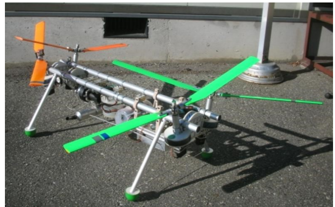
Figure 1 Intermeshing quadrotor helicopter.
