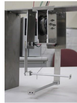
Figure 4 Angle measuring device with two potentiometer
