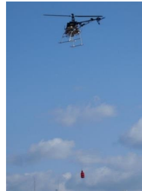
Figure 3 Flight test of a helicopter with a slung load system
