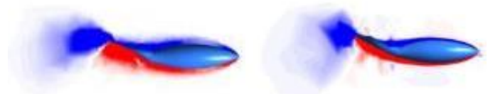
Figure 6 Vorticity-Y components, |\omega_Y| = 1 \text{ s}^{-1} , at V = 0.5 \text{ m/s} , f = 0.5 \text{ s}^{-1} and \theta = 20^\circ of the round rear fin-shape: flat (left) and cupping (right)
