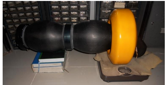
Figure 11 Center of Gravity Testing and measurement
