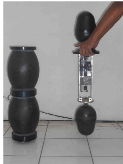
Figure 8 Buoyancy engine full assembly
