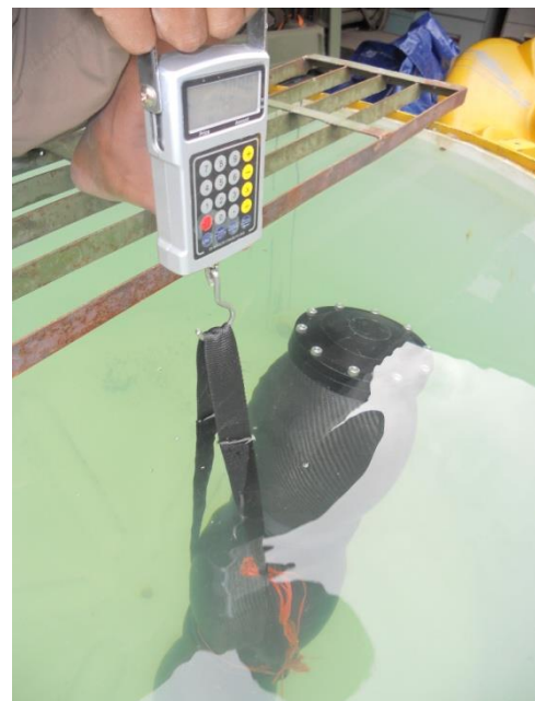
Figure 12 Static Bouyancy testing
