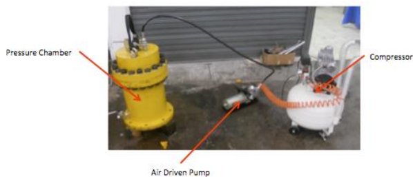
Figure 18 Testing Setup with Pressure Chamber
