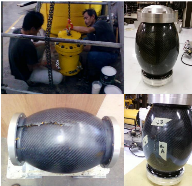
Figure 12 The testing setup of composites modular dry box (top), Crush test until maximum pressure the specimen can hold it (Bottom).
