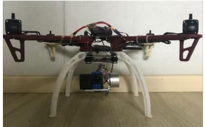
Figure 1 DJI F450 Quadcopter with Firefly 7s camera
