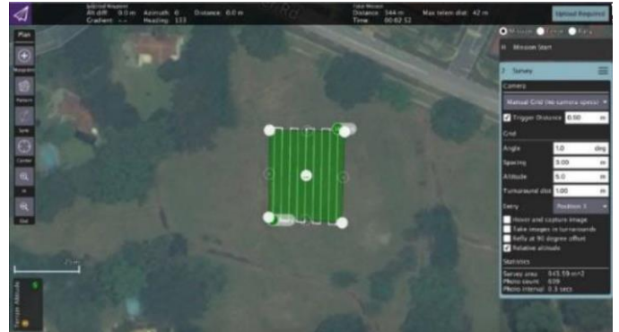
Figure 2 Waypoints set in QgroundControl as flight path
