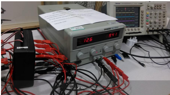
Figure 11 Power supply and PWM Generator
