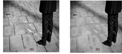
Figure 16 Amplification of the masked area (a) without median filter (b) with median filter
