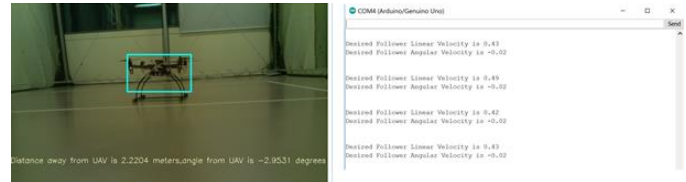
Figure 22 (a) Success detection of UAV with the corresponding distance and angle (b) Line formation output the desired velocities to maintain formation.
