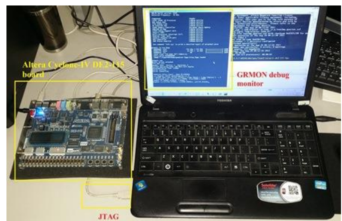
Figure 8 Debugging LEON3 processor
