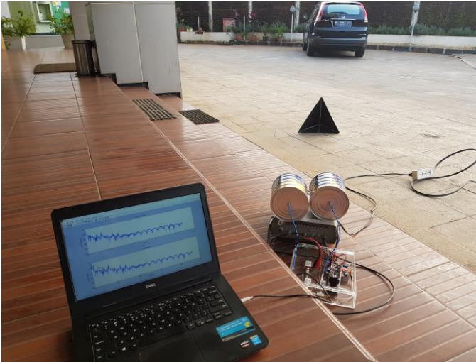
Figure 11 Real ground testing using corner reflector
