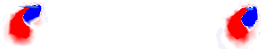
Figure 7 Vorticity-Y components, |\omega_Y| = 1 \text{ s}^{-1} , in a root plane and St = 1.95 : lunate profile (left), rectangular profile (right). (Blue: negative vorticity, Red: positive vorticity)
