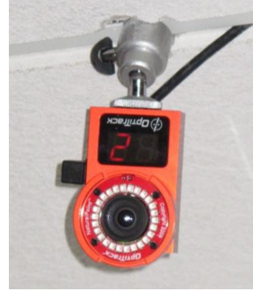
Figure 5 V100:R2 camera used for Optitrack positioning system
