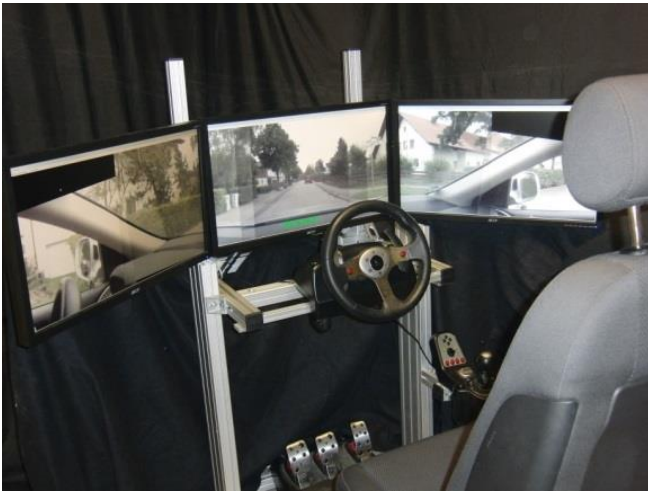
Figure 1 The simulator used for this experiment is also used for real world test drives
