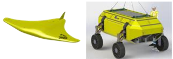
Figure 3 Underwater glider for deep-sea application (left). Underwater crawler from MOVES-Seismic design team for seismic and electromagnetic measurements at the seafloor (right)
