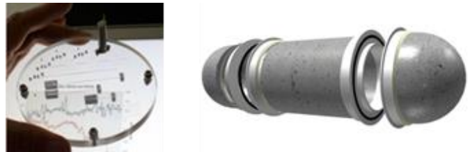
Figure 5 Lab-on-chip (LOC) technology (left). Concrete housing for underwater application (right)
