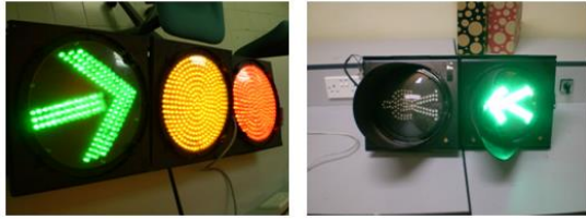
Figure 2 LED traffic light (left) and LED pedestrian light (right) are under testing in lab
