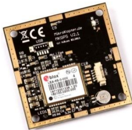
Figure 10 GPS module ( MK GPS v2.1 ) from Mikrokopter
