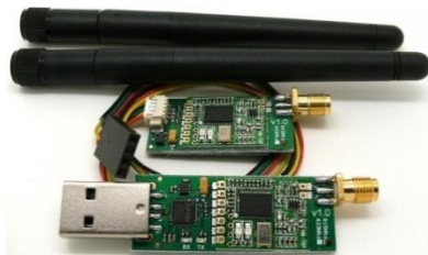
Figure 11 UAV's data transceiver from RCTimer
