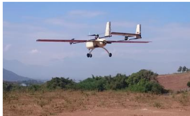
Figure 1 VTOL UAV for Aerial Surveillance Mission (Hadi, 2016)
