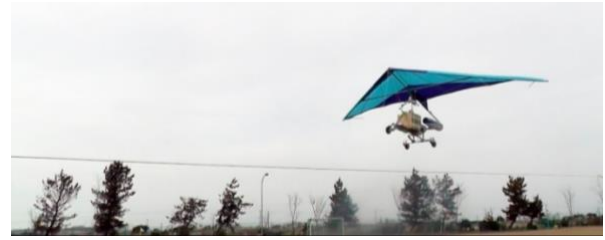
Fig 2 Safety flight testing of a cargo UAV at AIST (Iwata, 2013)
