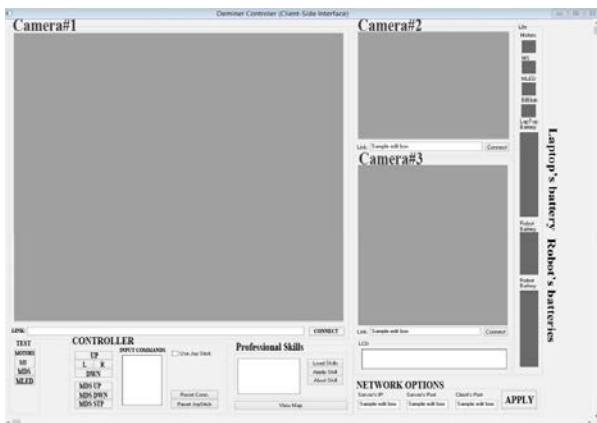
Figure 2 Operator GUI that contains camera monitoring, robot controller, and a mine illustrate, network monitoring, robot's batteries status illustrates, and laptop's battery status illustrates, motors statuses indicators
