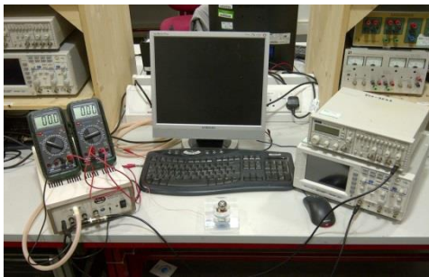
Figure 13 Practical test rig arrangement used to measure the characteristics of the fabricated USM actuator prototype using single flexural vibration transducer
