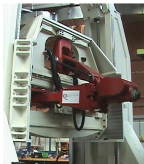
Figure 2 Physical model of the 5-DOF Exechon machine developed in Queen's University Belfast
