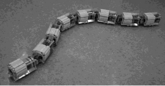
Figure 1 Overview of AMMR. The robot can be operated on ground and under water. In this paper, we considered the motion on ground
