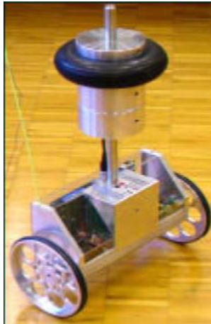
Figure 3 JOE: A mobile inverted pendulum
