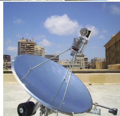
Figure 22 Calibration of counter weight and actuator testing
