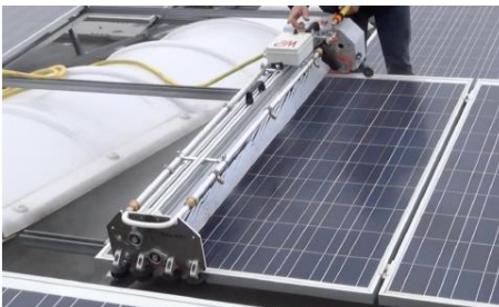
Figure 35 An example of a "Wash Panel" system [51]
