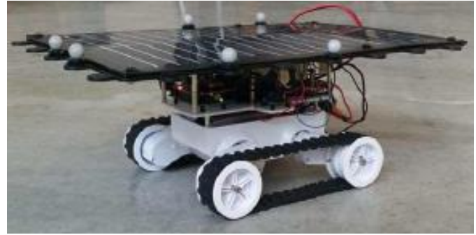
Figure 57 Demonstration vehicle with 18 W solar panel [163]
