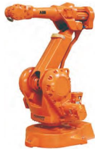
Figure 19 A modern six-axis robot from ABB [70]
