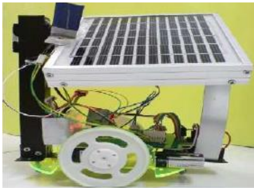
Figure 39 The solar tracker robot and solar panel
