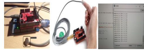
Figure 7 Body temperature sensor integrated to the ALT platform solution and setup
