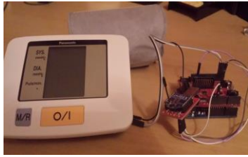
Figure 4 Blood pressure monitor setup connection and interface to the ALT platform solution
